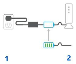
Unplug the battery from the power supply and the gateway.
